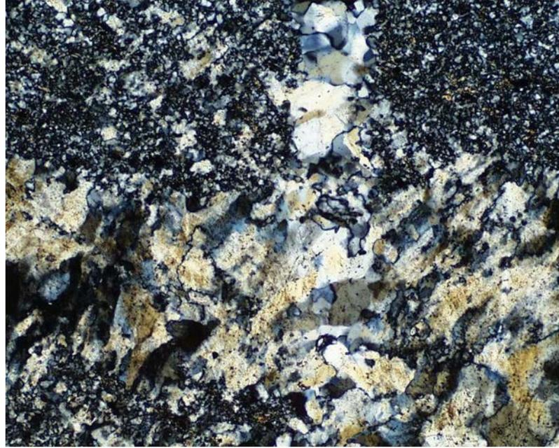
Figure 7: Photomicrograph of sample REB-148-1750 showing feathery quartz in a veinlet juxtaposed against fine grained quartz and sericite replacement of the primary rock matrix. 50X magnification, XPL.
