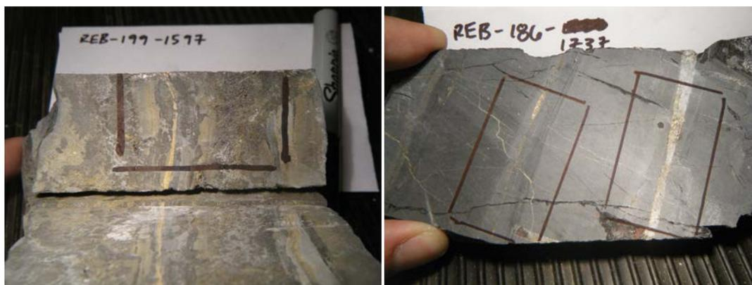
Figure 17: Two hand samples from core of pyrite morphology at the Mike deposit, associated with Carlin type mineralization and gold. Left: REB-199-1577 showing sooty disseminated sulfide in decarbonatized and lightly clay altered rock. Right: REB-186-1737 sulfide stringers parallel to bedding and small pyrite-carbonate veinlet parallel to bedding, possibly hydrothermal in origin.
