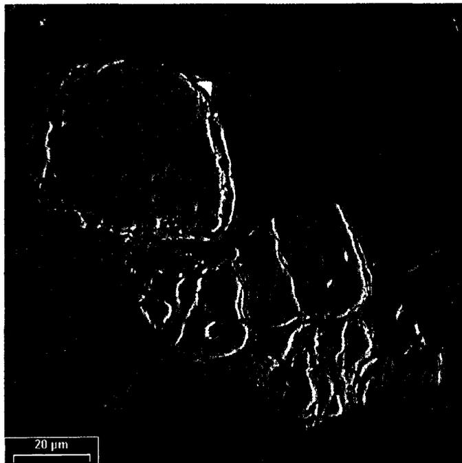
Figure 14. LC07ZJ156 SEM image of 2 gold blebs on rim of hematite pseudomorph after pyrite.
