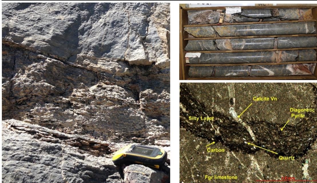
Figure 8. Notch Peak Formation A. Exposure of a siltstone bed between two beds of limestone. B. Drill core of light gray limestone. C. Photomicrograph (crossed polars) of silty layer in fine-grained limestone.
