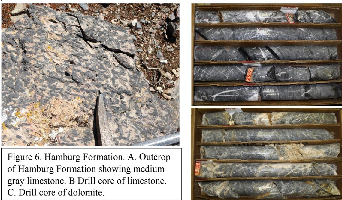
Figure 6. Hamburg Formation. A. Outcrop of Hamburg Formation showing medium gray limestone. B. Drill core of limestone. C. Drill core of dolomite.
