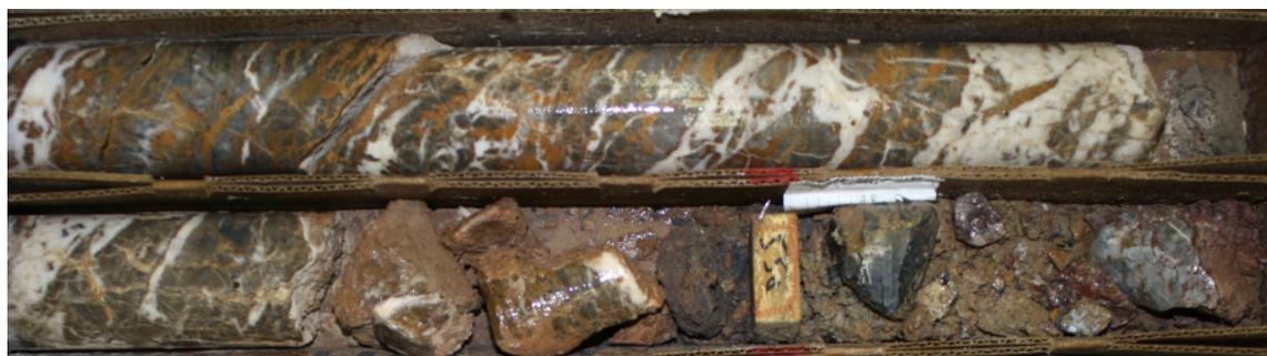
Figure 52. Drill core from Hamburg Limestone showing brecciated jasperoid veined by milky white quartz. The interval shown contains 0.06 ppm Au, 71 ppm As, 2790 ppm Ag, 4670 ppm Cu, 385 ppm Ni, and 1800 ppm W (PK005C-547'-550').
