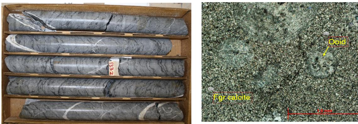
Figure 3. Geddes Limestone. A. Drill core showing light gray limestone with thin siltstone beds. B. Photomicrograph showing ooids (cross polars).
