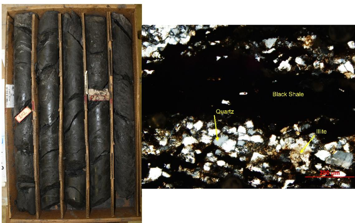
Figure 10. Pennsylvania black shale. A. Drill core. B. Photomicrograph showing interlayered carbonaceous shale and siltstone (quartz grains in illite matrix).
