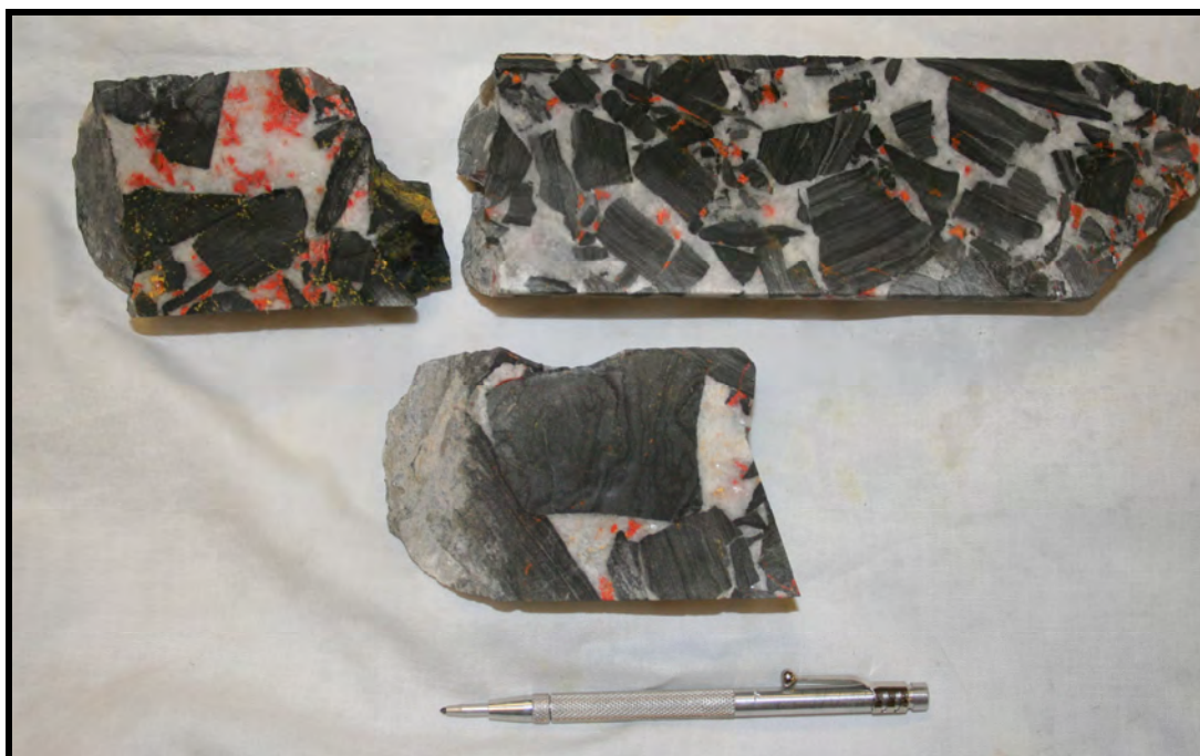
Figure 27. – Core from the Ruby Deeps orebody illustrating the more Carlin-type features of the system such as the dissolution/collapse breccias cemented by barite, calcite, and arsenic sulfides
