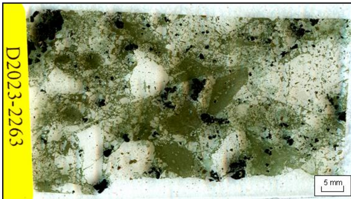
Figure 25. Scanned thin section of the breccia, showing the strong green color of the matrix (and biotite-altered clasts) that is due to the higher proportion of green biotite. Minor chlorite is present in the matrix as an alteration product of biotite. (D2023-2263').
