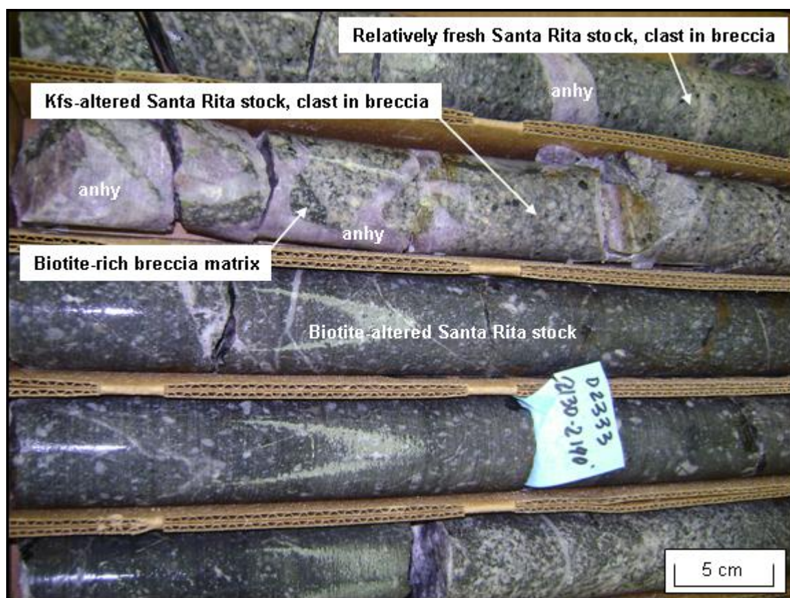
Figure 27. Purple anhydrite cutting various phases of the Santa Rita stock and breccia, the “anhydrite pseudo-breccia.” (D2333-2140’, NQ core).
