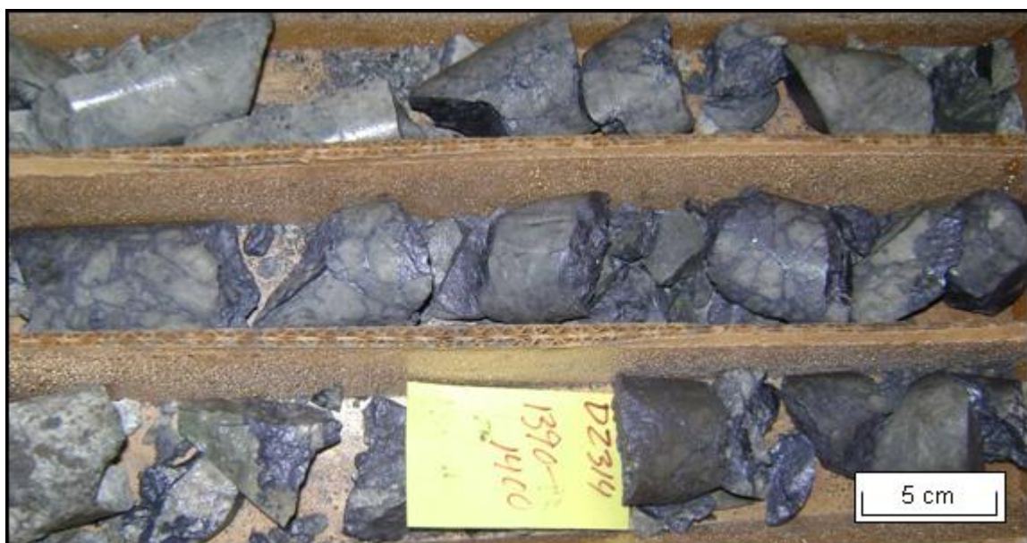
Figure 11. Molybdenite-cemented crackle breccia, assaying about 1% Mo. Clasts are mostly silicified rhyolite sill (D2314-1400').
