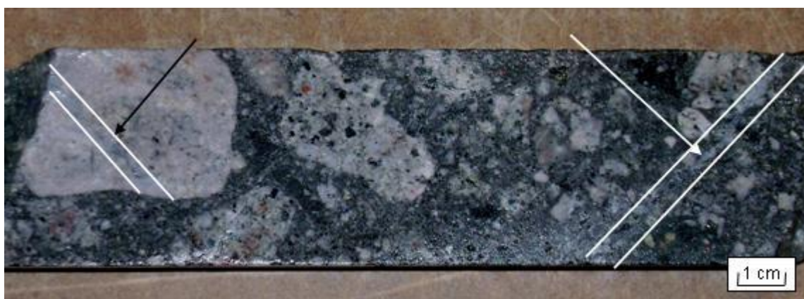
Figure 42. Evidence for two veinlet-controlled molybdenite mineralization events. There is a quartz-molybdenite veinlet that is truncated by the breccia matrix in the large leucocratic granite fragment in the left side of the picture (black arrow), and a quartz-molybdenite veinlet that cuts the matrix on the right side (white arrow). This interval assays 0.046% Mo, in veinlets (D2156-2241', NQ core).
