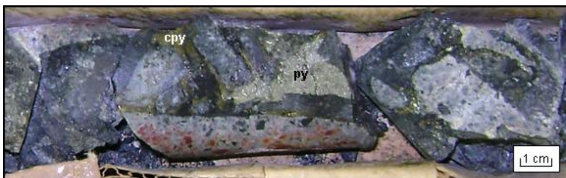
Figure 46. Core photograph showing the strong chalcopyrite (cpy) and pyrite (py) with chlorite in the breccia matrix (D2039-1550', NQ core).
