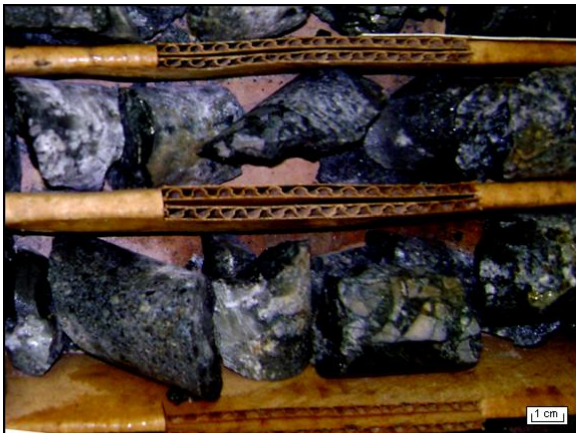
Figure 26. Core photograph of the breccia near the location of the previous thin section, showing the deep green color of the matrix (D2023-2220') (NQ-sized core).
