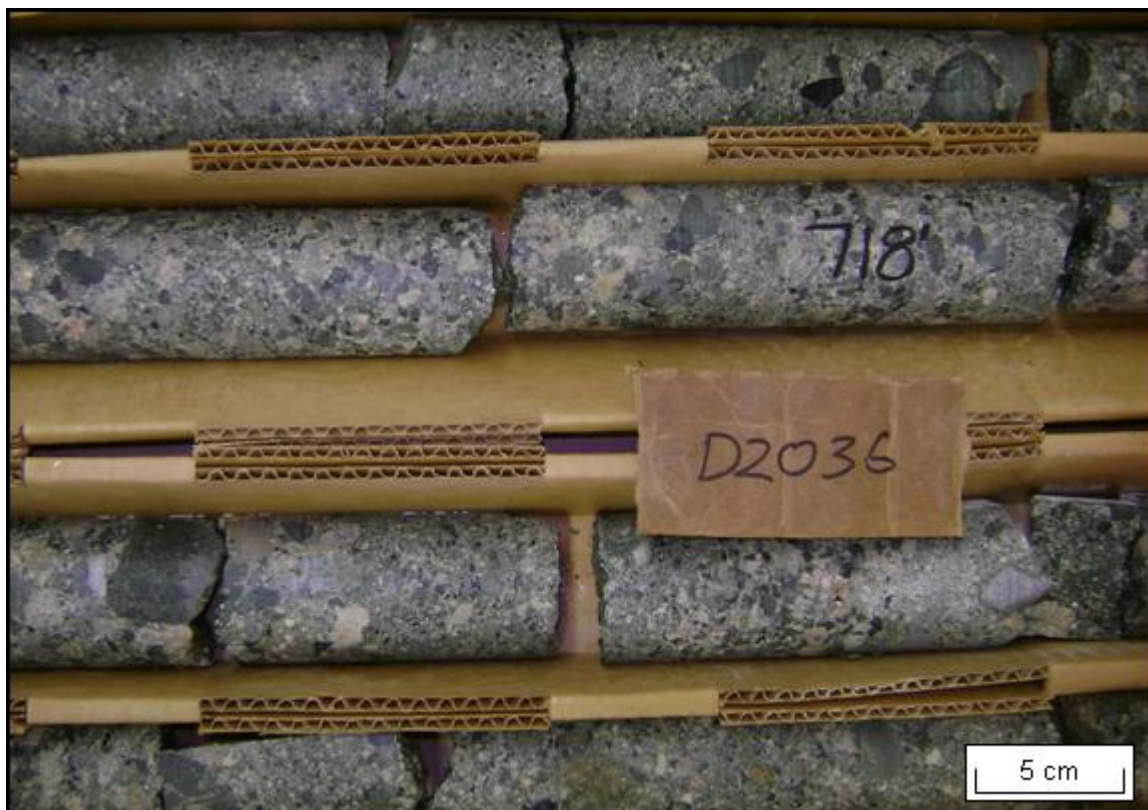
Figure 10. Hanover Hole diatreme breccia, showing the extreme clast type variation, and changes in matrix:clast ratio (D2036-718', NQ core).
