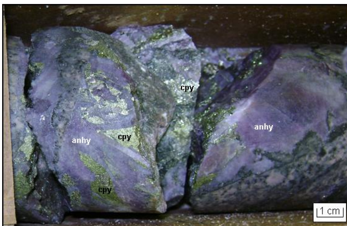
Figure 49. Core photograph of the massive anhydrite (anhy) with chalcopyrite (cpy) (D2333-1735', HQ-sized core).
