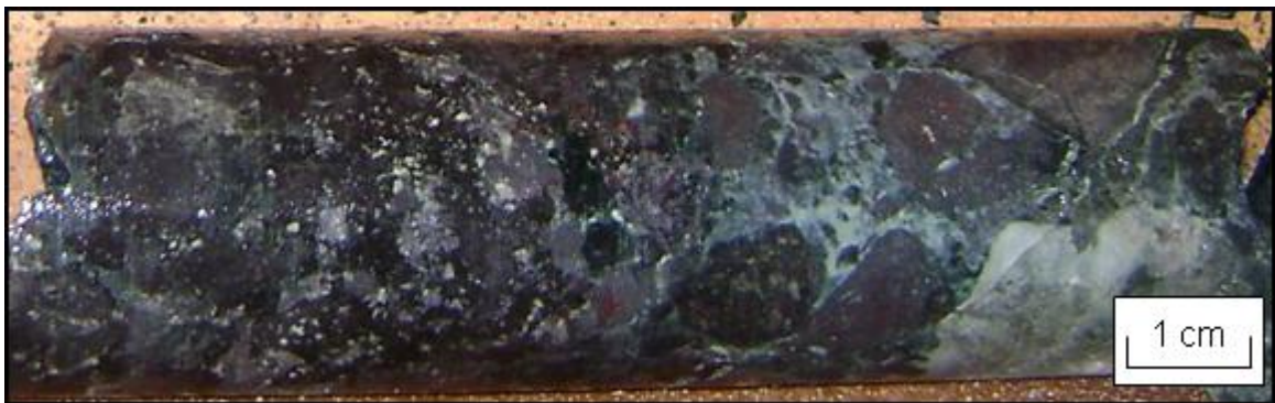
Figure 29. Core photograph of brecciated prograde skarn. Magnetite-rich clasts in matrix dominated by serpentine, talc, and chlorite. The lighter-colored serpentine-talc matrix on the right side of the photo overprints the darker, chlorite-dominated matrix in the left side of this piece (D2314-1620') (NQ core).
