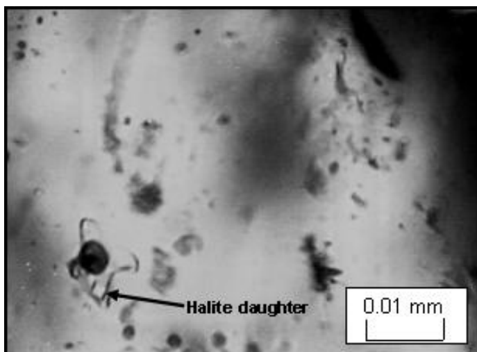
Fig 63. Rare halite-saturated fluid inclusion that homogenized below 500°C (D2329-1374-2, 1a, Th = 482°C, Th(halite) = 215°C).
