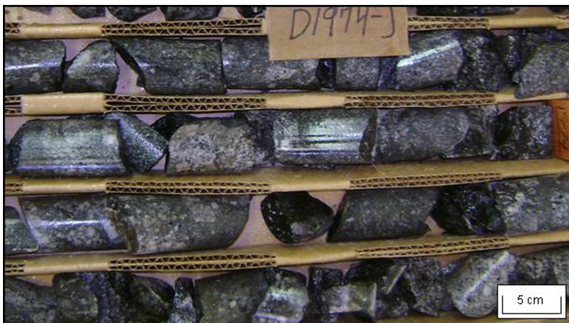
Figure 15. Core showing the “intrusive breccia,” from which the thin section in Figure 16 was made (D1974, 2804-2796’, NQ core).
