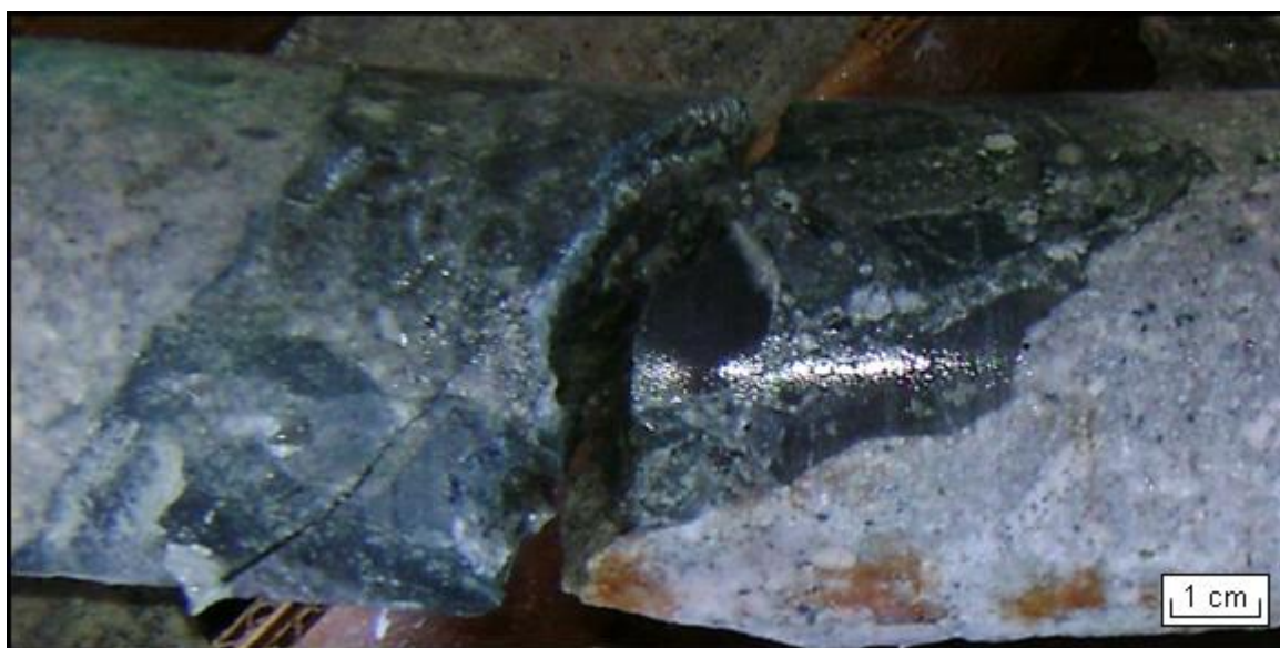
Figure 31. Core photograph of biotite- and chlorite- rich breccia as a clast in pseudo-porphry breccia, which is the matrix on either side of the breccia clast. (D2332-2004') (HQ-size core).
