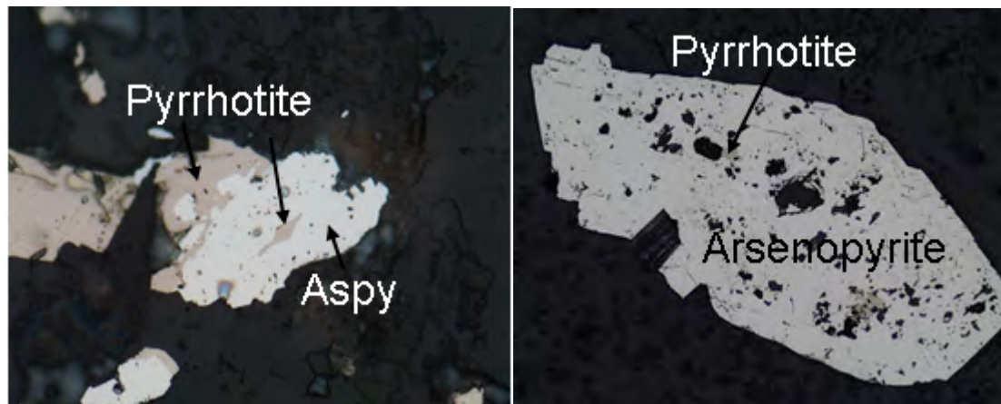
Figure A 20. Replacement of pyrrhotite by arsenopyrite both located to the north of Dome, left FOV = 0.43, reflected light; right FOV = 2.2mm, reflected light.
