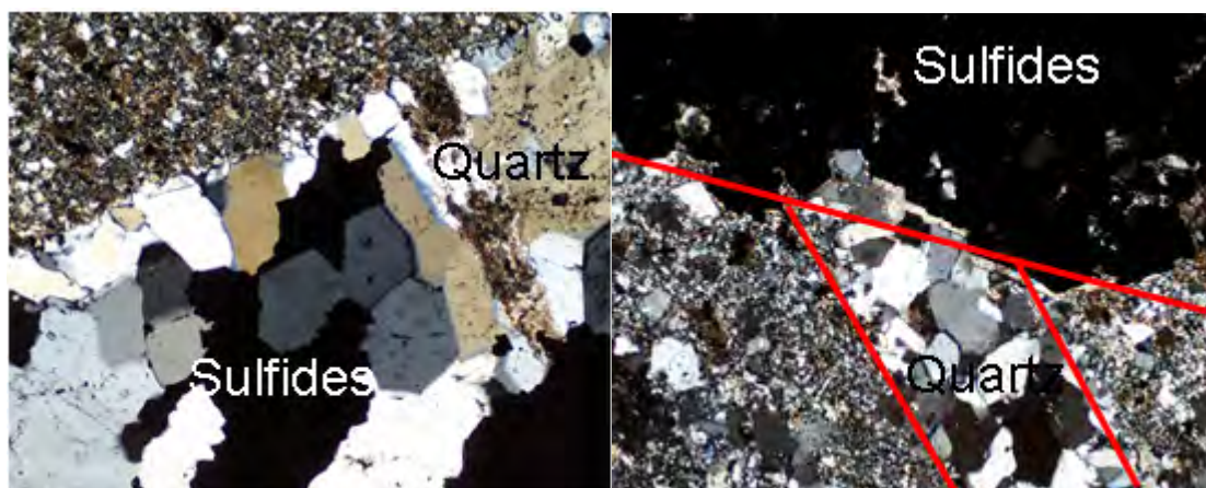
Figure A 9. A sugary textured quartz vein with sulfides filling in between grains and overprinting this phase found to the north and east of Dome, both FOVs are 4.4mm and XPL.
