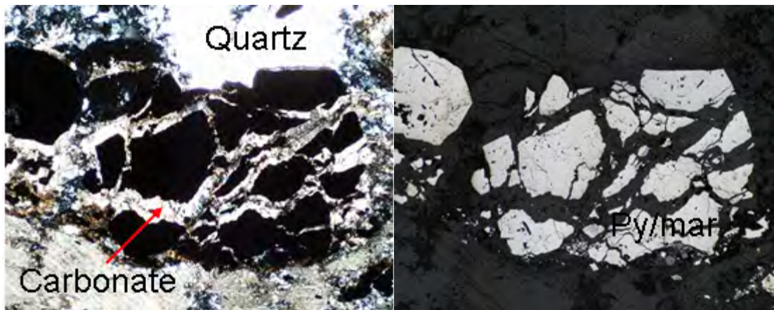
Figure A 15. Carbonate phase that broke up pyrite and marcasite grains in the Quartz district, FOV = 4.4mm, XPL and reflected light.
