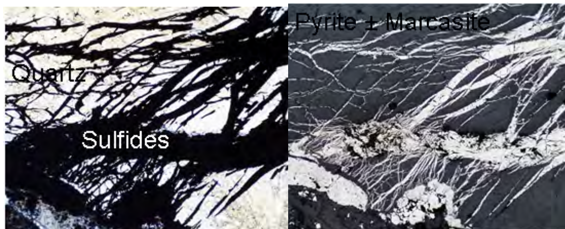
Figure A 8. Large groundmass quartz grain overprinted by pyrite and marcasite in the Quartz district, FOV = 4.4mm, left = XPL, right = reflected light.
