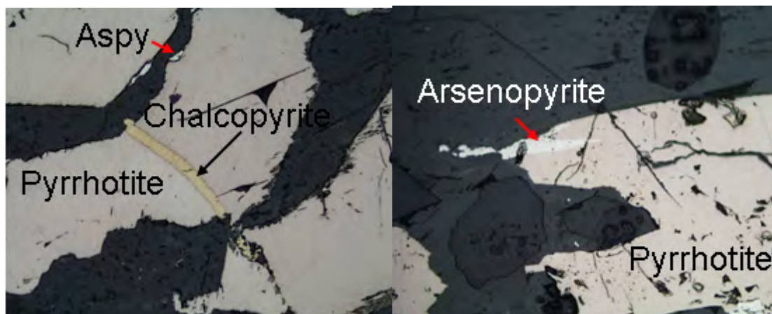
Figure A 18. Left: chalcopyrite overprinting pyrrhotite and the formation of arsenopyrite at the grain boundary found north of Dome, FOV = 1.1mm, reflected light.
