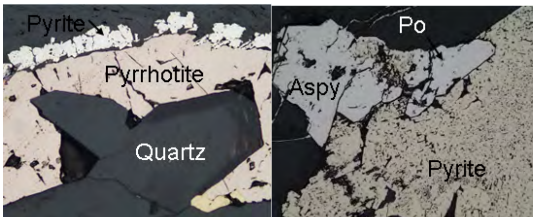
Figure A 22. Left: pyrrhotite grains that formed between euhedral quartz grains. Pyrite formed at the opposite pyrrhotite grain boundary, FOV = 1.1mm, reflected light.
