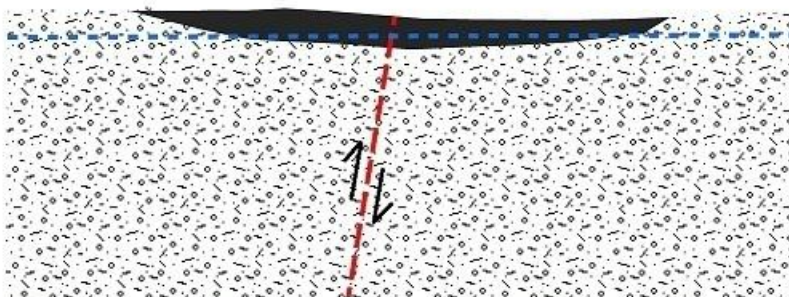
Figure 40 – Theoretical depositional model for vein – type manganese
