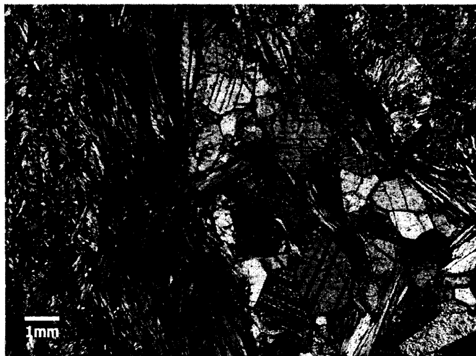
Figure 34. Photomicrograph of actinolite schist showing fine-grained actinolite and carbonate, crossed Nicols, 2 mm field of view. Same sample as above.
