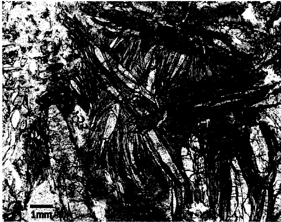
Figure 71a. Silica-carbonate alteration, early stages. Photo field of view 2 mm, plane light.
