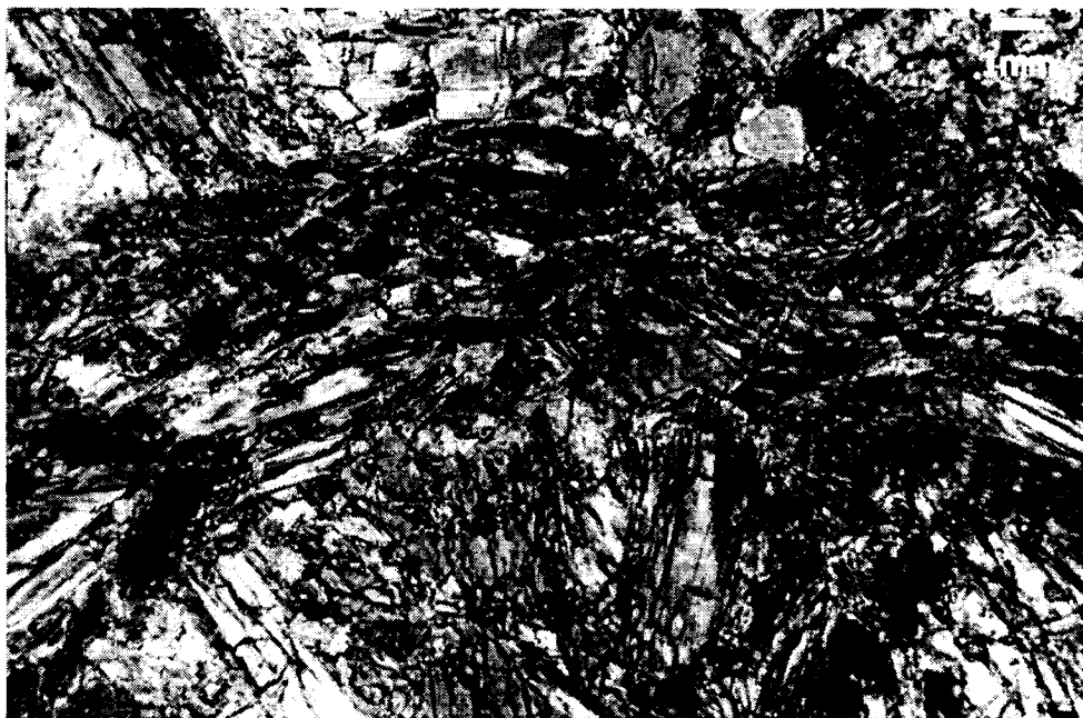
Figure 42. Photomicrograph of biotite-amphibole-garnet schist. Field of view is 1.33 mm, crossed Nicols.
