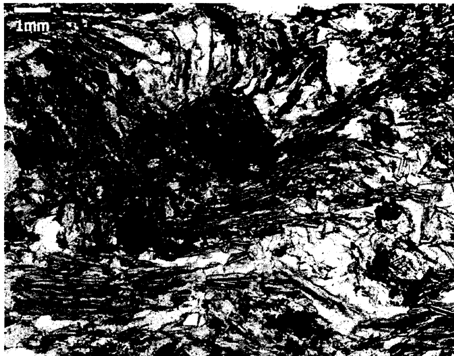
Figure 47. Graphite folded with biotite (bleached) and quartz (plane light, field of view 2 mm, sample 200703-2).
