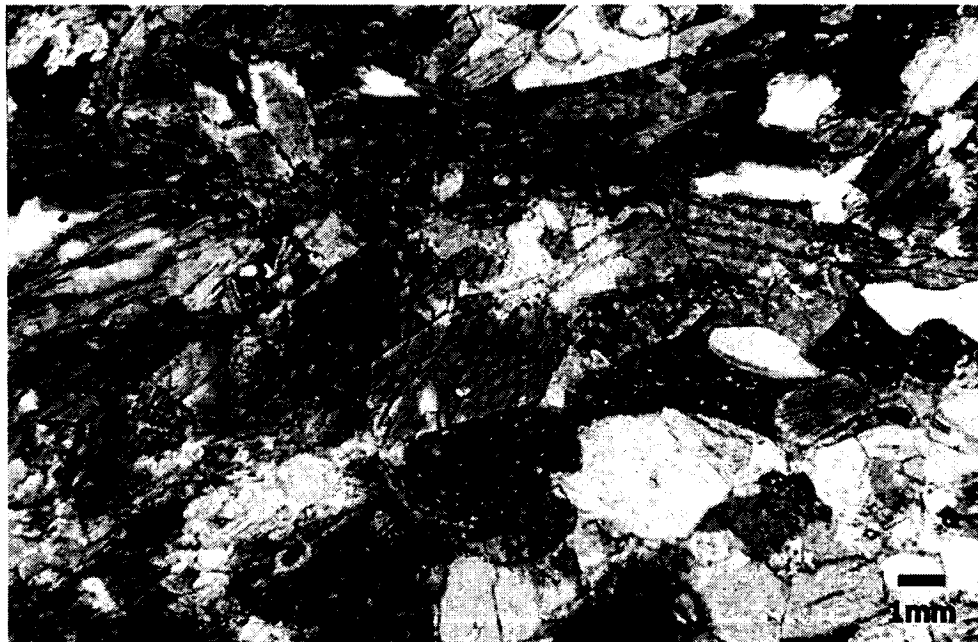
Figure 51. Photomicrograph of sample 060802-4 showing crudely aligned hornblende, biotite, and calcite. Field of view is 1.33 mm, crossed Nicols.
